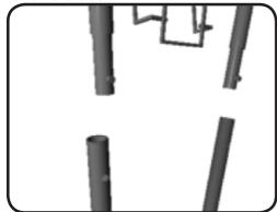
Place the top section onto the bottom section, making sure that it snaps into place.
