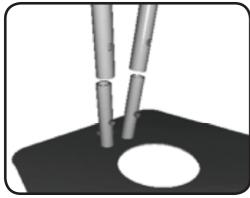
Place the bottom section onto the foot, making sure that it snaps into place. Make sure the narrow end is down.
